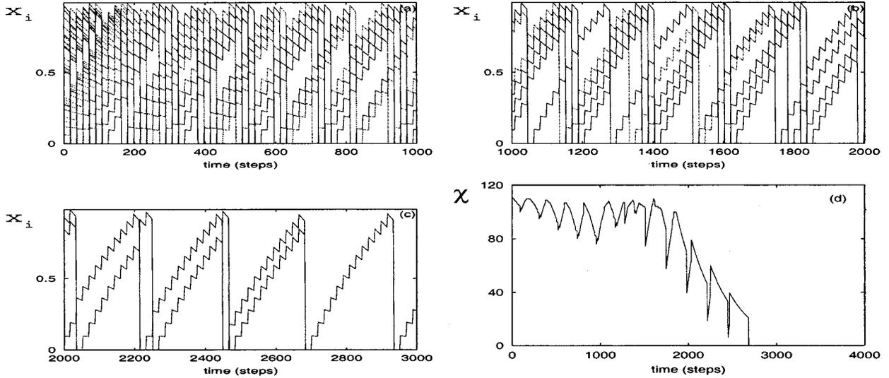
FIG. 1. (a), (b), (c) Behavior of 30 excitable LIF neurons coupled by spikes. In the following, we denote by step the time unit for integrating Eq. (6). External inputs are periodic with period  $T=18$  (steps) and intensity  $\bar{\epsilon}=0.1$ . The coupling strength is  $\epsilon=0.007$ , and the decay rate is  $\gamma=0.003$  (step) $^{-1}$ . (d) Behavior of the synchronization parameter  $\chi(t)$  of the same time series.
