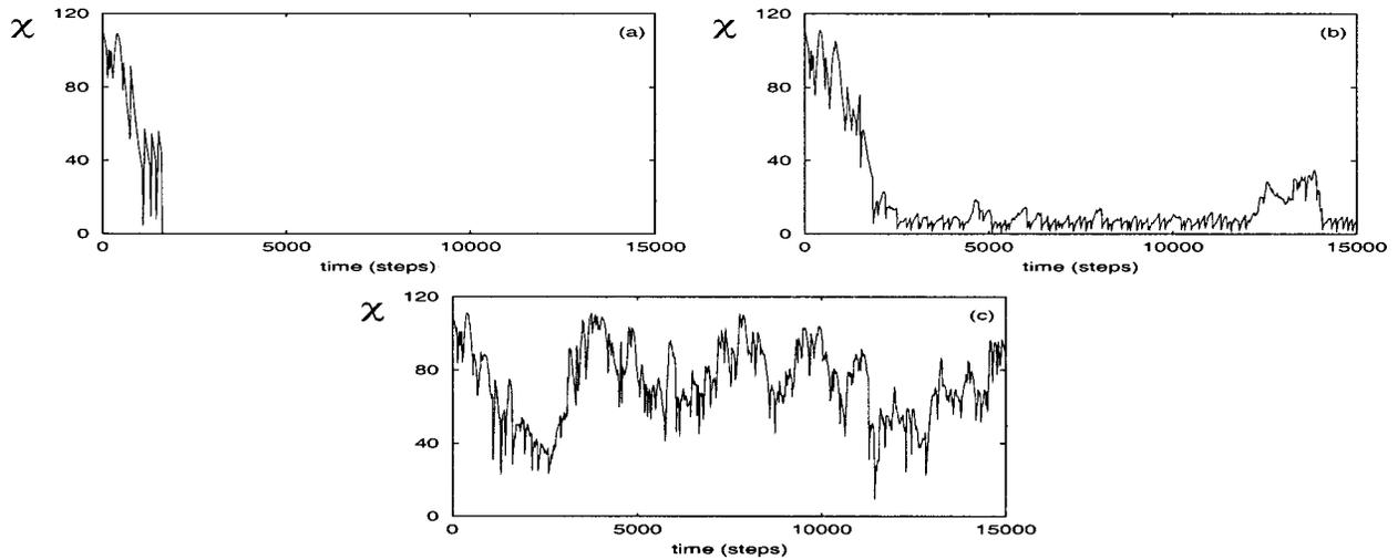
FIG. 2. Behavior of the synchronization parameter  $\chi(t)$  of 30 excitible LIF neurons coupled by spikes.  $\bar{\epsilon}=0.18$ ,  $\epsilon=0.005$ , and  $\gamma=0.003$  (step)<sup>-1</sup>. Interspike intervals of external inputs have probability density  $\rho(t)=e^{-0.04t}/0.04$  (step)<sup>-1</sup>. White noise intensity is  $\sigma=0$  (step)<sup>-1</sup> (a),  $\sigma=0.003$  (step)<sup>-1</sup> (b), and  $\sigma=0.009$  (step)<sup>-1</sup> (c).
